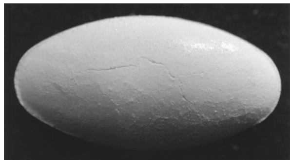
Figure 1. Longitudinal crack on the upper side of a mefenamic acid tablet.
